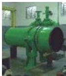
Butterfly Valve 40" with by-pass for Small Hydroeletric plant ENERG POWER
